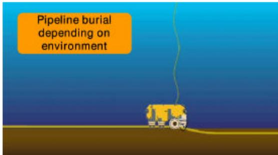
Deep sea pipelines are normally laid on top of the seabed allowing it to embed in the seabed under its own weight, except in near-shore areas, where it is physically buried in order to minimize the effects of human activity and protect the pipeline from sea currents and storms. An automated robotic trenching machine lifts the laid pipe, digs the trench where the pipeline is to be lowered, and refills it with a layer of excavated soil/rock and sand after the pipeline burial.
