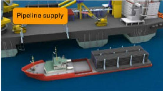
Each pipe section for Medgaz pipeline is normally **12 meters** long, with a **24-inch (610 mm)** diameter. For mechanical protection and corrosion resistance, these pipes are to be manufactured with a triple-layer coating: first layer consisting of epoxy resins, a second made out of adhesive material and a third made of polypropylene for anti-abrasion properties. For shallower water depth areas, a concrete coating will also be added to give increased protection from fishing gears.
