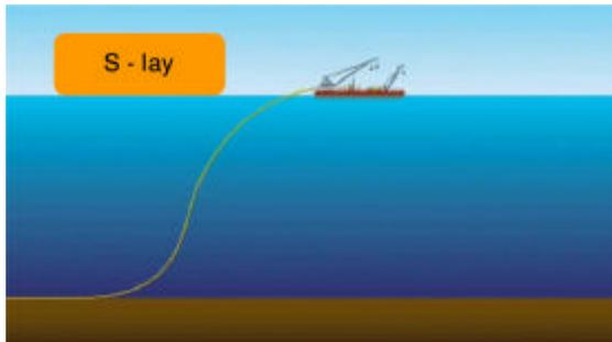
Pipe lay Barge system will be used to build the offshore portion of the pipeline, which consists of a mobile platform or barge where the pipeline is welded before being laid on the seabed in a continuous fashion.
