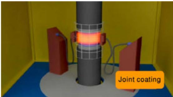
During this finishing procedure, the exposed welded joints are coated with two layers, one made of epoxy resin and the other of polypropylene to maintain continuity with the rest of the pipe.
