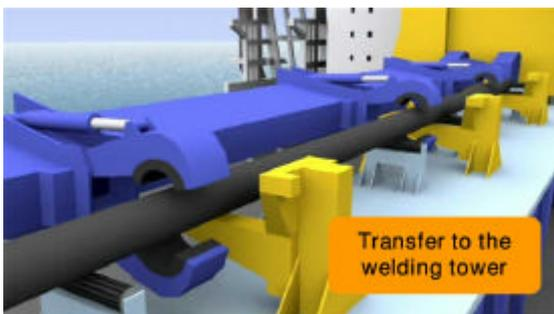
The pipe sections are placed in the middle of the platform and using grippers and rollers raised up to the welding tower, where they are to be welded together at the girth joint using submerged arc welding equipment.
