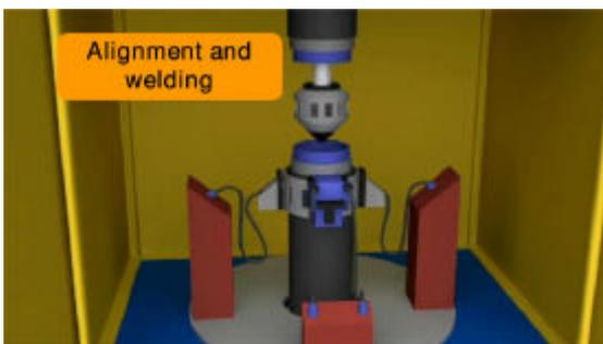
The pipes are aligned in the tower and welded by automated welding machineries. In order to do so, the platform holds tight the part of the submerged pipeline being welded onto, while at the top, new pipe sections arrive that are then joined by welding and undergo the following quality control and finishing processes.
