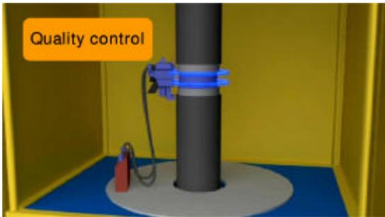
Each welded joint is individually tested by non destructive techniques (NDT) and verified by inspectors using advanced quality control techniques before being certified to be fit for subsequent finishing processes.
